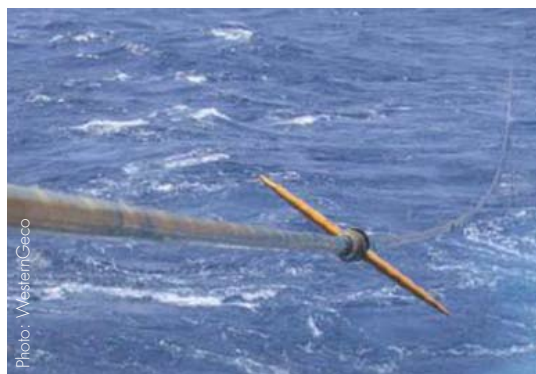
The steering devices (yellow birds) used to control both depth and lateral position of the streamer.
